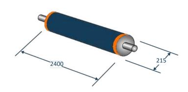
It is recommended to leave 100-150 mm of free space between the part and the tank walls for adequate ultrasonic diffusion.
